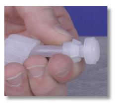
**Step 34:** If the tube nut is not securing, recheck the ferrule connection. Pull the tube nut toward the nozzle, once more, to compress the collar and nozzle together. Retighten the tube nut until secure.
