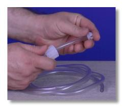
**Step 108:** Slide the collar back onto the tube, and make sure the collar's crown is pointing away from the tube nut.
