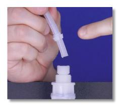
**Step 146:** Slide the collar back onto the tube, and make sure the collar's crown is pointing away from the tube nut.
