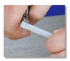
**Step 10:** Look at the end of the tube. If the tube's end is flared, use the diagonal pliers to cut the flared portion off.
