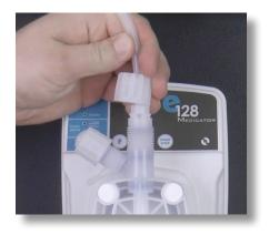
**Step 141:** Reattach the tube, and tube connections onto the discharge valve by hand tightening the tube nut. Do not cross thread nor overtighten.
