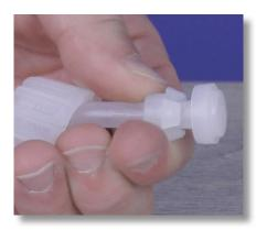
**Step 150:** Always be mindful of the orientation for the tubing connections. First is the tube nut, followed by the collar and nozzle.
