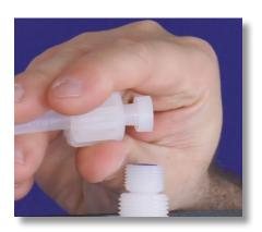
**Step 32:** Pull the tube nut toward the nozzle to compress the collar and nozzle tight together. This should form a ferrule connection.
