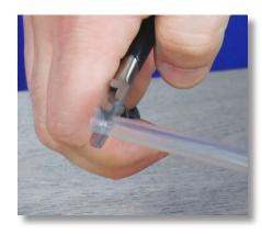
**Step 48:** Look at the end of the tube. If the tube's end is flared, use the diagonal pliers to cut the flared portion off.
