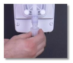
**Step 111:** Reattach the tube, and tube connections onto the suction valve by hand tightening the tube nut. Do not cross thread nor overtighten.
