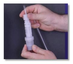
**Step 63:** Loosen the foot filter tube nut and disconnect the PVC suction tubing, tube nut, collar, and nozzle attached.
