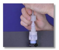
**Step 100:** Reattach the tube, and tube connections onto the injection valve by hand tightening the tube nut. Do not cross thread nor overtighten.
