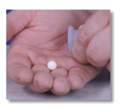
**Step 118:** Pour the ceramic ball out of the filter seat and into your hand. Set the filter seat down and use the small towel to wipe the ceramic ball clean. Do not misplace it.
