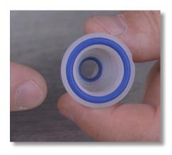
**Step 42:** While holding onto the ceramic ball, inspect the two blue o-rings in the grooves of the filter seat and make sure they are not damaged.
