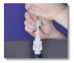
**Step 143:** Loosen the injection valve tube nut and disconnect the discharge tubing along with the tube nut, collar, and nozzle attached.
