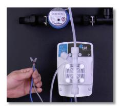
**Step 156:** If the issue continues, inspect the connection to the water meter to see if it is loose or disconnected.
