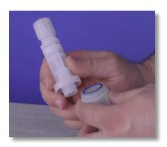
**Step 38:** The filter seat may stick to the filter body. Make sure it rests in the filter basket instead, to avoid losing the ceramic ball.
