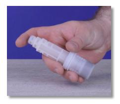
**Step 37:** Shake the foot filter back and forth. You should hear a ceramic ball moving freely inside. If not, separate the foot filter into three (3) pieces by popping the filter basket from the filter body.
