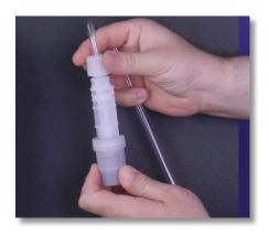
**Step 128:** Grab the foot filter and reattach the tube, and tube connections onto the foot filter by hand tightening the tube nut. Do not cross thread nor overtighten.
