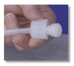
**Step 13:** Pull the tube nut toward the nozzle to compress the collar and nozzle tight together. This should form a ferrule connection.
