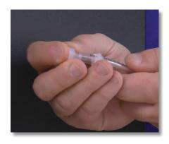
**Step 77:** Slide the nozzle back into the tube's opening. Push the collar and nozzle together as close as possible.
