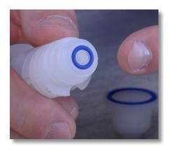
**Step 71:** Grab the filter body and inspect to make sure the small blue o-ring on the top of the filter body is not damaged.
