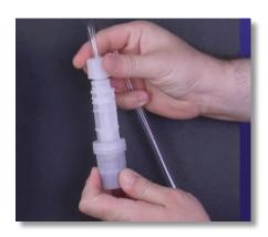
**Step 51:** Grab the foot filter and reattach the tube, and tube connections onto the foot filter by hand tightening the tube nut. Do not cross thread nor overtighten.
