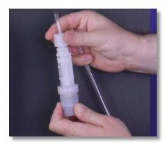
**Step 113:** Loosen the foot filter tube nut and disconnect the PVC suction tubing, tube nut, collar, and nozzle attached.
