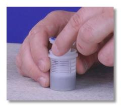
**Step 72:** Set the filter body down, grab the filter basket and put the filter seat back into the filter basket.
