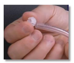
**Step 76:** Slide the collar back onto the tube, and make sure the collar's crown is pointing away from the tube nut.
