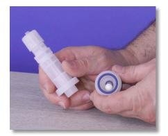
**Step 66:** Set the filter body aside and locate the ceramic ball in the filter seat.
