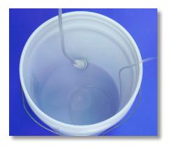
**Step 81:** Place the foot filter back into the chemical bucket or stock tank, making sure it is sitting vertically.
