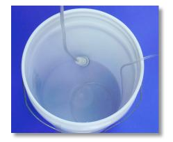
**Step 130:** To finish up, look at the PVC suction's tube condition. If the tube is cracked, rigid, or looks really old replace it now.
