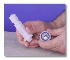
**Step 116:** Set the filter body aside and locate the ceramic ball in the filter seat.
