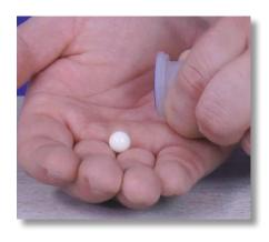
**Step 68:** Pour the ceramic ball out of the filter seat and into your hand. Set the filter seat down and use the small towel to wipe the ceramic ball clean. Do not misplace it.
