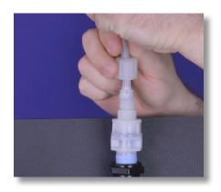
**Step 95:** Disconnect the discharge tubing along with the tube nut, collar, and nozzle attached.
