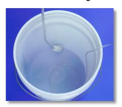
**Step 35:** Inspect the foot filter by taking it out of the chemical bucket or stock tank.
