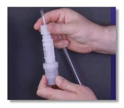
**Step 36:** Loosen the foot filter tube nut and disconnect the PVC suction tubing, tube nut, collar, and nozzle attached.
