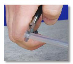
**Step 124:** Look at the end of the tube. If the tube's end is flared, use the diagonal pliers to cut the flared portion off.
