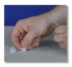
**Step 74:** Grab the PVC suction tubing hanging down from the suction valve. Remove the nozzle and collar from the tube and set aside. Do not lose them.
