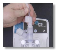
**Step 93:** Reattach the tube, and tube connections onto the discharge valve by hand tightening the tube nut. Do not cross thread nor overtighten.
