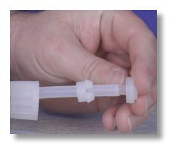
**Step 89:** Inspect your tubing connections by removing the nozzle, and collar from the tube and set aside. Do not lose them.
