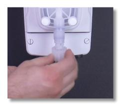
**Step 24:** Reattach the tube, and tube connections onto the suction valve by hand tightening the tube nut. Do not cross thread nor overtighten.
