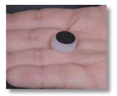
**Step 17:** Check to see if the black transit washer is stuck to the nozzle and remove.
