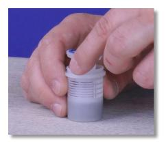
**Step 121:** Set the filter body down, grab the filter basket and put the filter seat back into the filter basket.
