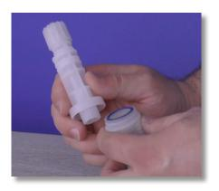
**Step 115:** If not, separate the foot filter into three (3) pieces by popping the filter basket from the filter body.
