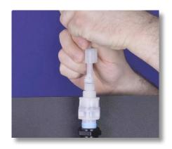
**Step 27:** Loosen the injection valve tube nut and disconnect the discharge tubing along with the tube nut, collar, and nozzle attached.
