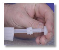
**Step 12:** Slide the nozzle back into the tube's opening. Push the collar and nozzle together as close as possible.
