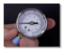
**Step 134:** Assess if the pressure of the installation is too high by using a pressure gauge.
