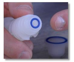
**Step 120:** Grab the filter body and inspect to make sure the small blue o-ring on the top of the filter body is not damaged.
