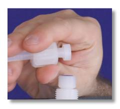
**Step 148:** Pull the tube nut toward the nozzle to compress the collar and nozzle tight together, forming a ferrule connection.
