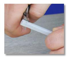
**Step 145:** Look at the end of the tube. If the tube's end is flared, use the diagonal pliers to cut the flared portion off.
