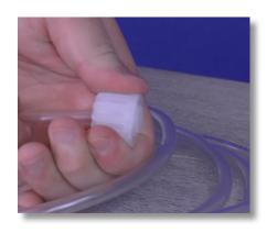
**Step 110:** Pull the tube nut toward the nozzle to compress the collar and nozzle tight together, forming a ferrule connection.
