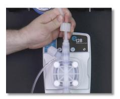
**Step 6:** To check the discharge valve, loosen the discharge valve tube nut and lift the discharge tube, tube nut, collar and nozzle attached.
