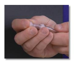
**Step 126:** Slide the nozzle back into the tube's opening. Push the collar and nozzle together as close as possible.
