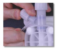
**Step 60:** Slide the bleed-off tubing back onto the air bleed barb.
