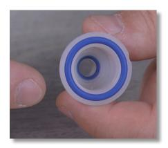
**Step 119:** While holding onto the ceramic ball, inspect the two blue o-rings in the grooves of the filter seat and make sure they are not damaged. Put the ceramic ball back into the filter seat and set the filter seat aside.
