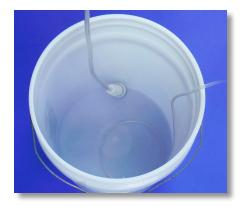
**Step 53:** Place the foot filter back into the chemical bucket or stock tank, making sure it is sitting vertically.
