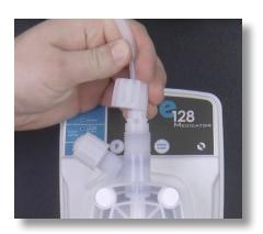
**Step 14:** Reattach the tube, and tube connections onto the discharge valve by hand tightening the tube nut. Do not cross thread nor overtighten.
