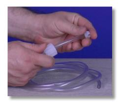
**Step 21:** Slide the collar back onto the tube, and make sure the collar's crown is pointing away from the tube nut.
