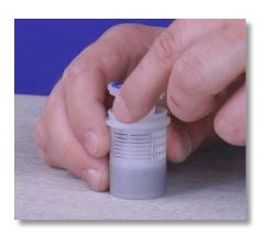
**Step 67:** Pull the filter seat out of the filter basket and set the filter basket aside.
