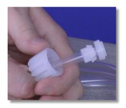
**Step 80:** Always be mindful of the orientation for the tubing connections. First is the tube nut, followed by the collar and nozzle. Make sure the collar's crown is pointing away from the tube nut.
