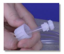
**Step 129:** Always be mindful of the orientation for the tubing connections. First is the tube nut, followed by the collar and nozzle.
