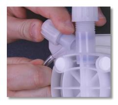
**Step 83:** Remove the bleed-off tubing from the air bleed barb and set aside.
