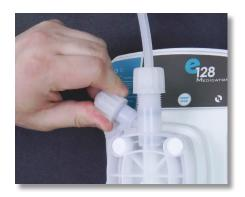
**Step 86:** Now close the air bleed valve by turning it clockwise, and slide the bleed-off tubing back onto the air bleed barb.
