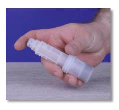
**Step 64:** Let the tubing hang from the pump head while you inspect the foot filter. Shake it back and forth. You should hear a ceramic ball moving freely inside.
