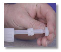
**Step 139:** Slide your nozzle back into the tube's opening. Push the collar and nozzle together as close as possible.
