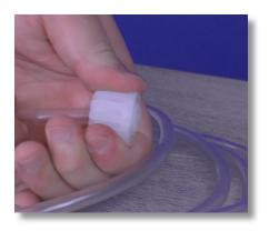
**Step 23:** Pull the tube nut toward the nozzle to compress the collar and nozzle tight together. This should form a ferrule connection.
