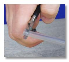
**Step 107:** Look at the end of the tube. If the tube's end is flared, use the diagonal pliers to cut the flared portion off.
