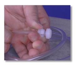
**Step 25:** If the tube nut is not securing recheck the ferrule connection. Pull the tube nut toward the nozzle, once more, to compress the collar and nozzle together. Retighten the tube nut until secure.
