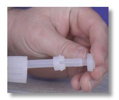
**Step 28:** Remove the nozzle and collar from the tube and set aside. Do not lose them.
