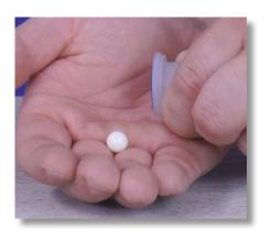
**Step 41:** Pour the ceramic ball out of the filter seat and into your hand. Set the filter seat down and use the small towel to wipe the ceramic ball clean. Do not misplace it.
