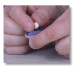
**Step 70:** Put the ceramic ball back into the filter seat and set the filter seat aside.
