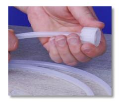
**Step 15:** If the tube nut is not securing recheck the ferrule connection.
