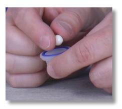
**Step 43:** Put the ceramic ball back into the filter seat and set the filter seat aside.
