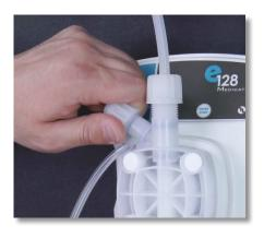
**Step 56:** Locate the air bleed valve on the upper left portion of the pump head and open it by turning the valve counter clockwise.
