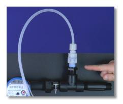
Once you have checked for the two transit washers, continue inspecting the tubing connections
