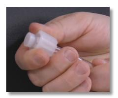
**Step 127:** Pull the tube nut toward the nozzle to compress the collar and nozzle tight together, forming a ferrule connection.
