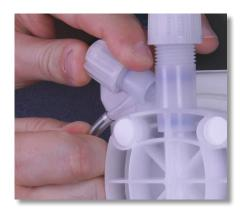
**Step 57:** Remove the bleed-off tubing from the air bleed barb and set aside.
