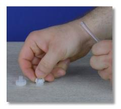
**Step 47:** Grab the PVC suction tubing hanging down from the suction valve. Remove the nozzle and collar from the tube and set aside. Do not lose them.
