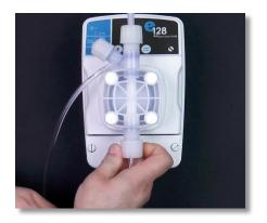
**Step 105:** Loosen the suction valve tube nut and disconnect the PVC suction tube, tube nut, collar, and nozzle attached.
