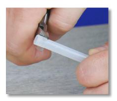
**Step 29:** Look at the end of the tube. If the tube's end is flared, use the diagonal pliers to cut the flared portion off.
